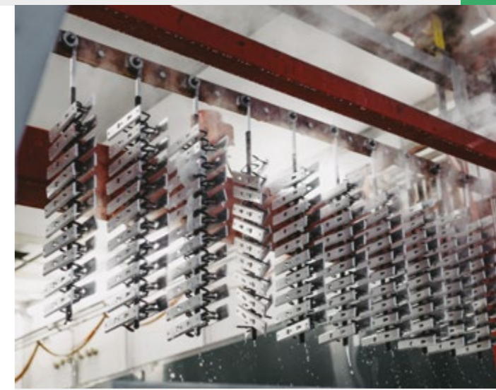
Colouring with the anodic oxidation method ensures longer product life; photo: AXA©.
